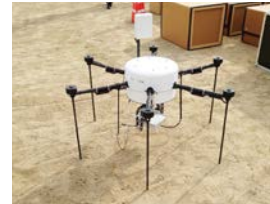
Drone relay station
