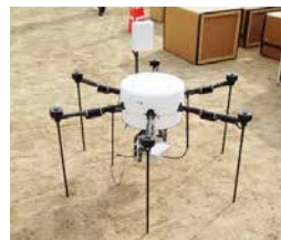
Drone relay station
