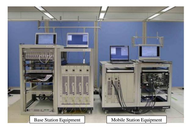
Note: In outdoor trials, the mobile station equipment will move around in a motor vehicle.
