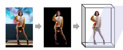
The system merges virtual performers with the real stage by projection onto a half-mirror film.
