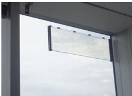
Glass antenna attached to an existing window
