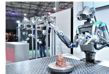
The remote-controlled robot, using “real haptics” technology and 5G, which enable tactile sensation information to be transmitted in real time, was displayed in the event. The feel of clay is fed back to the operator through the robot. The strengths of 5G, which include “low latency,” provide a stable telecommunication speed and have helped create many different machines.
