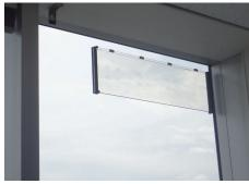
Glass antenna attached to an existing window
