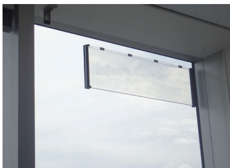
Glass antenna attached to an existing window
