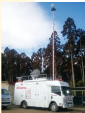
Equipment restored using satellite circuits
