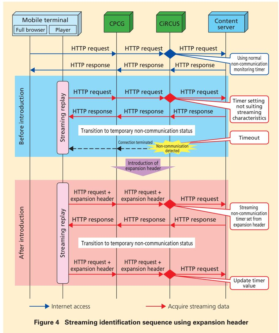
Figure 4 Streaming identification sequence using expansion header
