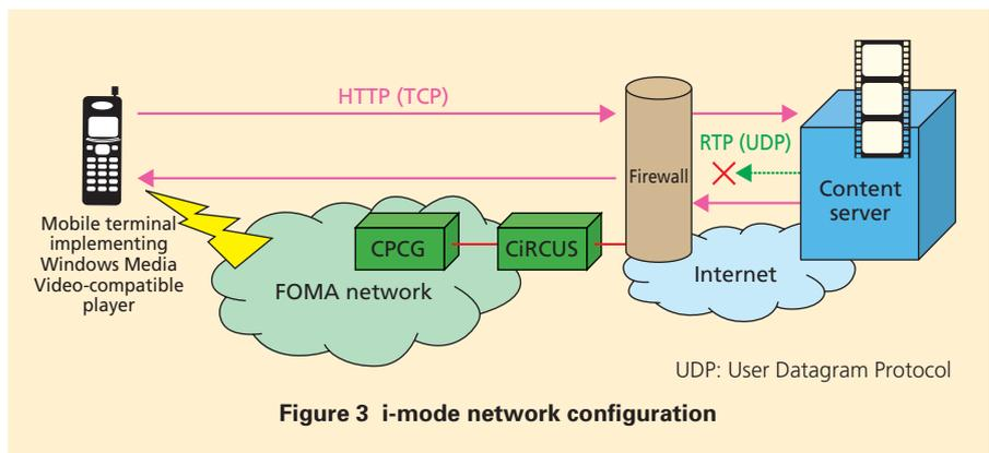
HTTP streaming adopts the HTTP method for streaming and performs encapsulation<sup>\*9</sup> of RTP packets with
