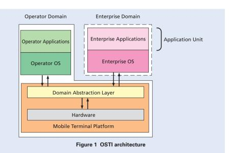
technologies. The OS Switching system exploits the suspend and resume functions found in many OSes to switch between two OSes in a mutually exclusive manner. The VMM, on the other hand, provides a set of virtual devices corresponding to the CPU, memory, and peripherals and has two OSes operate in parallel. The aim of DAL in the OSTI specification is to minimize the above differences.
