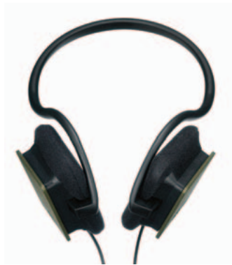
Photo 2 External view of headset with built-in antennas
