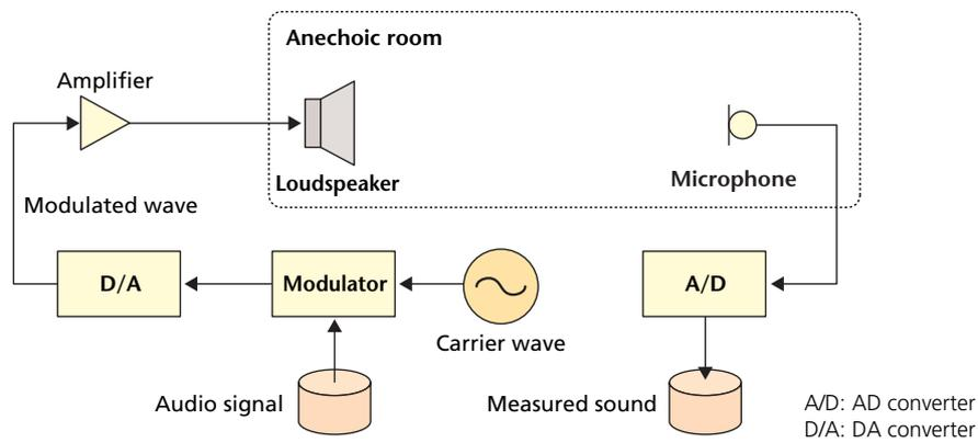
Figure 6 Measurement configuration
