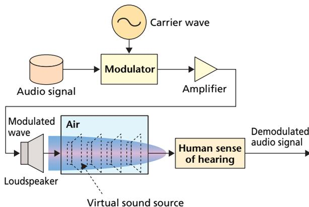
**Figure 1 Principle of super directional loudspeaker**
