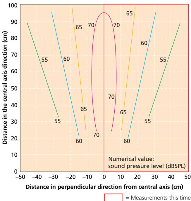
Figure 9 Sound pressure spatial distribution of demodulated wave (2 kHz)
