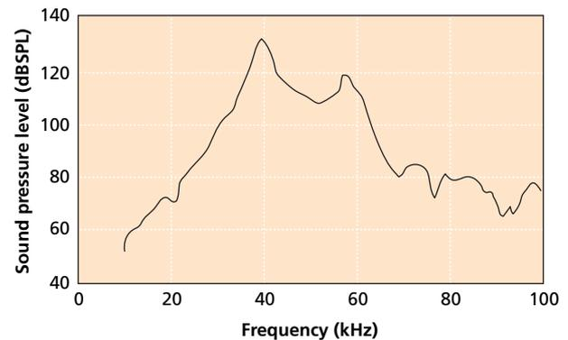
**Figure 5** Sound pressure frequency response of loudspeaker
