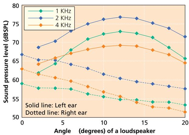
Figure 11 Angle of loudspeaker and sound pressure of demodulated wave
