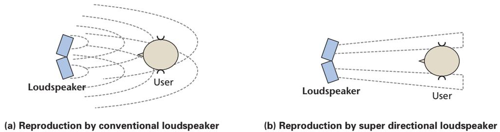
Figure 3 Sound reproduction for left and right ears using two loudspeakers mounted on mobile terminal
