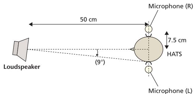
Figure 10 Placement of HATS and loudspeaker
