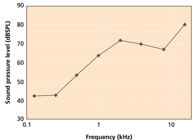
Figure 7 Sound pressure frequency response of demodulated wave
