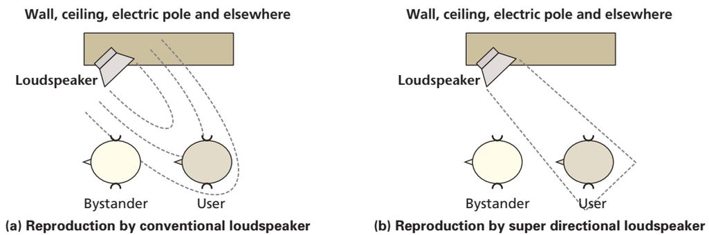
Figure 4 Sound reproduction toward moving user via external loudspeaker
