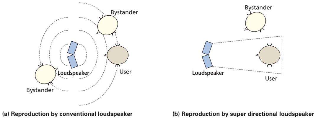
Figure 2 Sound reproduction by loudspeaker mounted on mobile terminal
