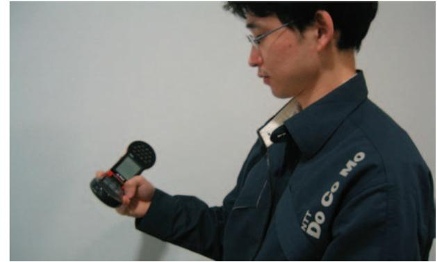
**Photo 1** Prototype of mobile super directional loudspeaker
