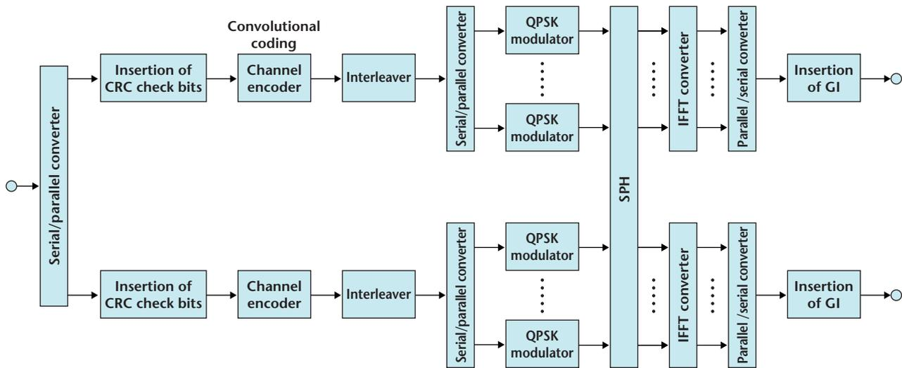
Figure 1 Configuration of MIMO-OFDM transmitter using SPH
