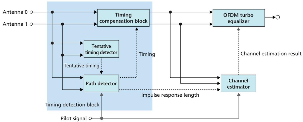
**Figure 4 Timing recovery method using high-precision path detector**
