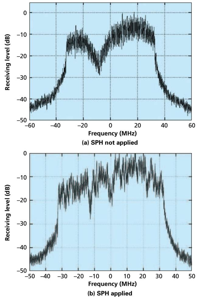
Figure 2 Spectrum with/without SPH
