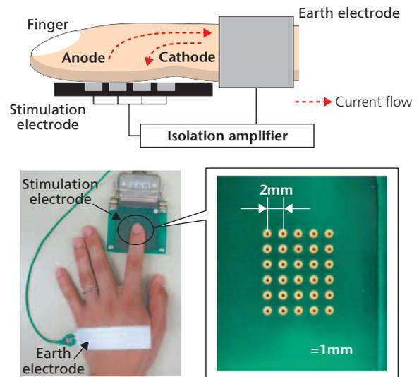
Figure 5 Configuration of electrocutaneous display
