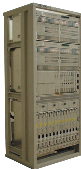
Photo 1 4-carrier 6-sector BTS (example)
