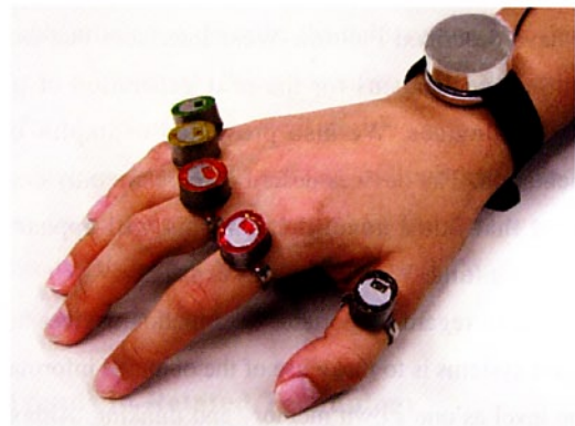
Photo 2 Fulltime-Wear Text Input Mechanism (FingerRing)
