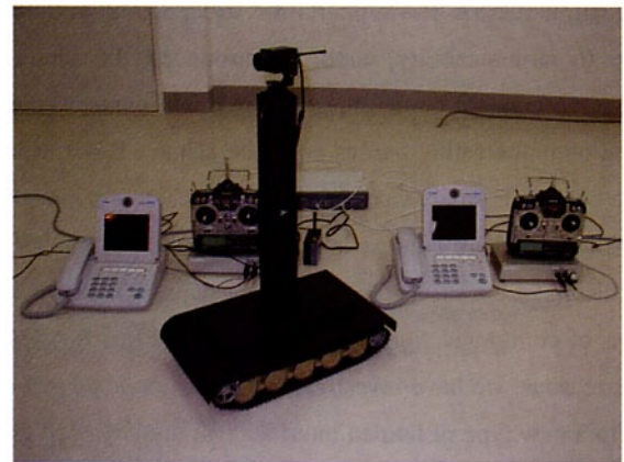
Figure 6 Experimental Mobile Robot for Remote Monitoring via Videophone
