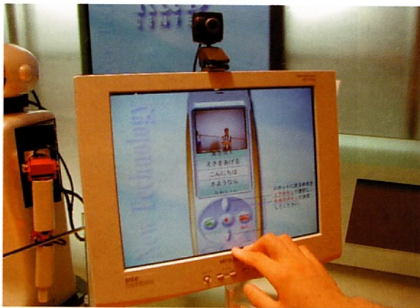
Figure 7 Virtual Terminal for Alter-Ego Robot Operation
