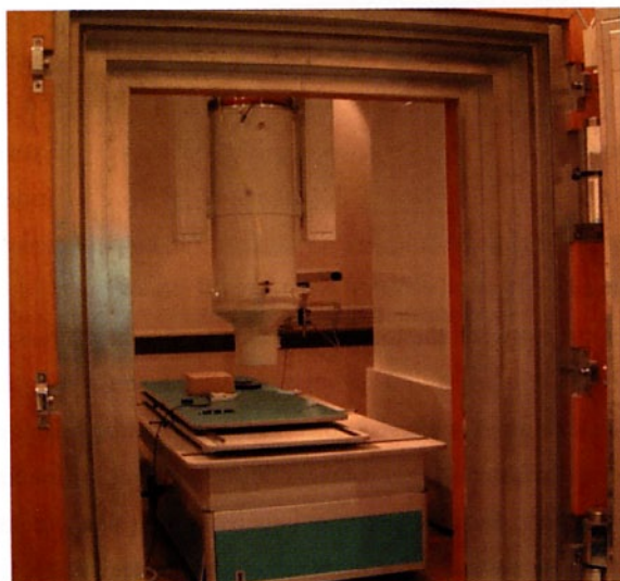
Photo 2 External Appearance of the SQUID Biomagnetic Measuring System (Seen from the entrance to the magnetically shielded room, the middle cylindrical object is the dewar)
