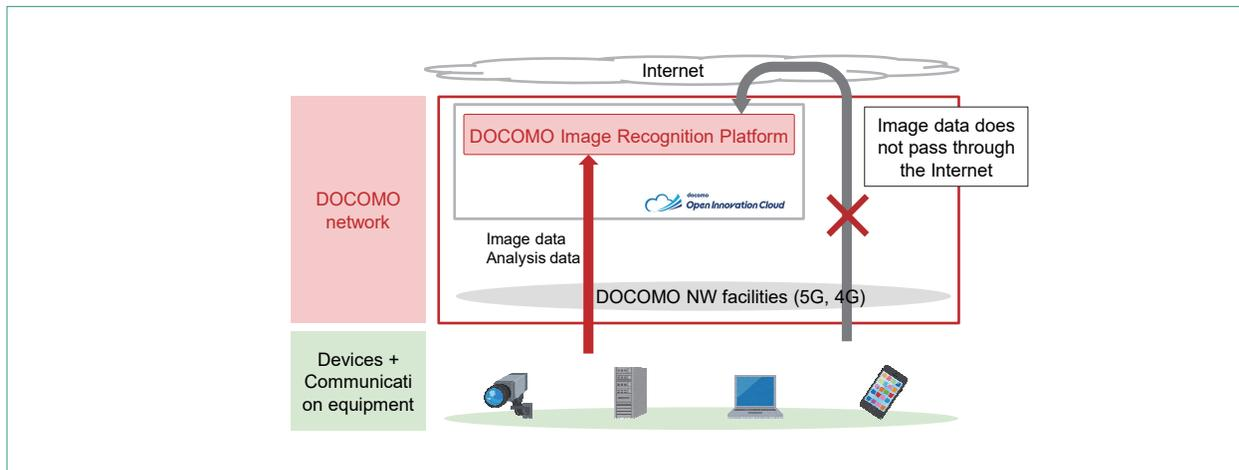
Figure 5 Using closed network connections to make image recognition secure
