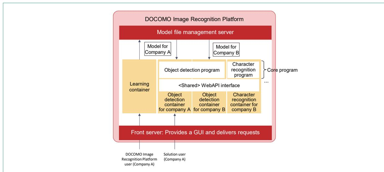
Figure 4 Using containerization to provide image recognition functions
