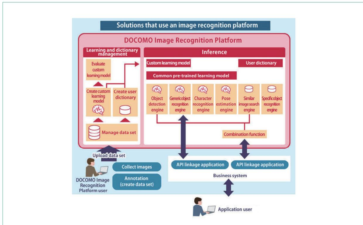
Figure 3 Functioning of the DOCOMO Image Recognition Platform
