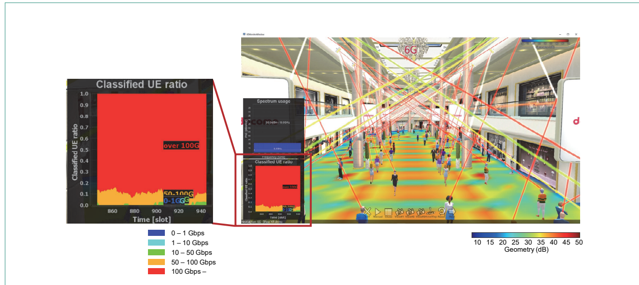
Figure 6 Evaluation results for 6G when adding IRSs and moving BSs (shopping mall)
