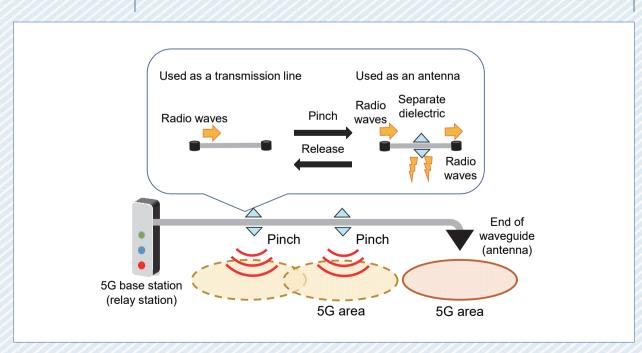
Technology Reports (Special Articles) Pinching Antenna—Using a Dielectric Waveguide as an Antenna— (P.5) Deploying a communication area with a bended antenna
