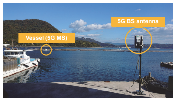
Photo 1 5G BS installed on land and 5G MS installed on the vessel
