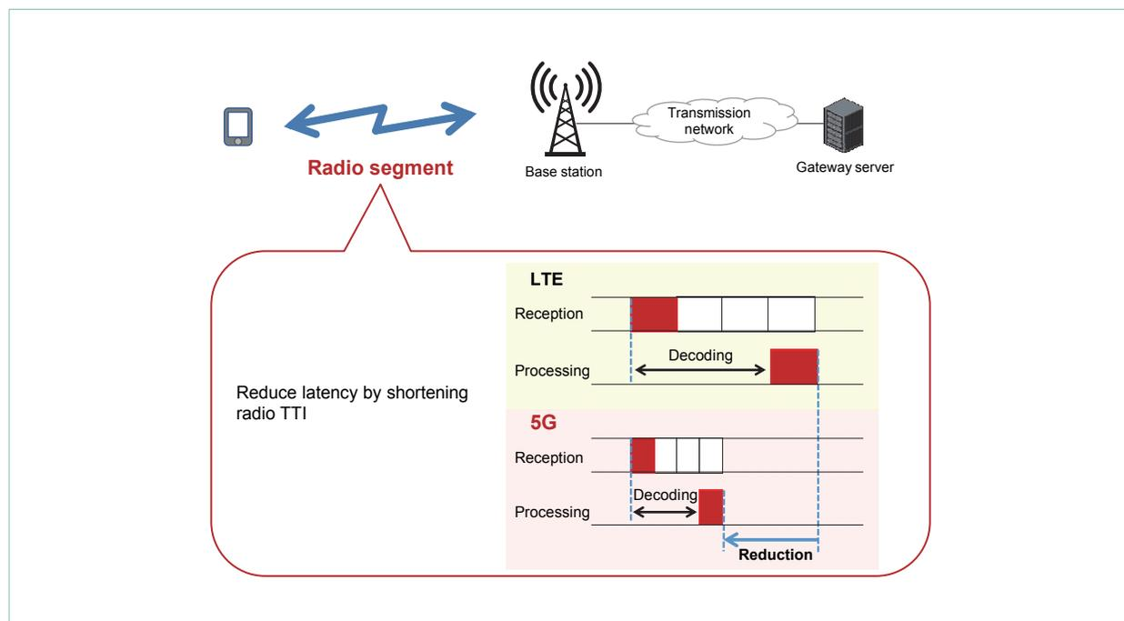
Figure 3 Reduction of latency on radio segment
