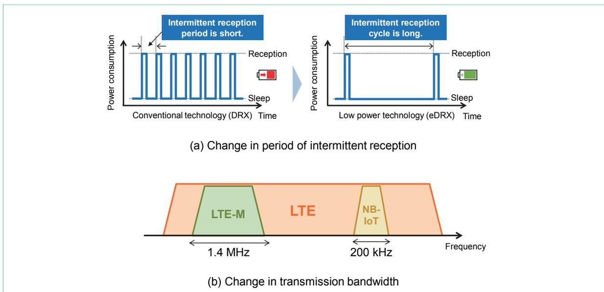
Figure 4 Low power consumption technologies
