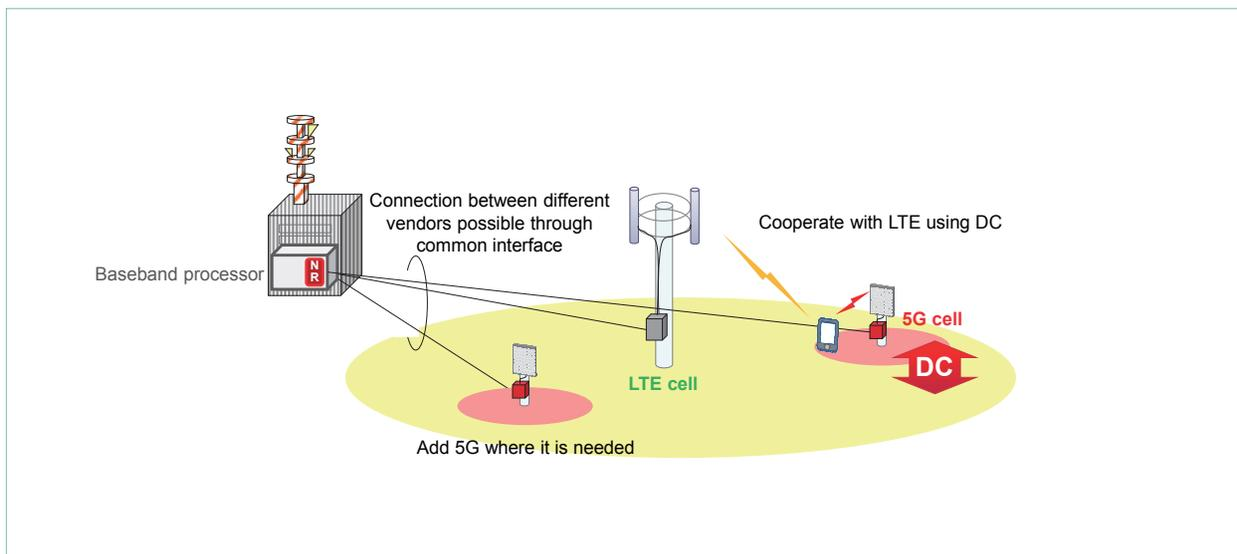
Figure 7 5G NSA deployment using DC
