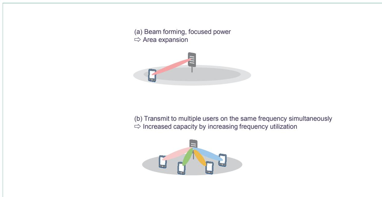
Figure 2 Massive MIMO
