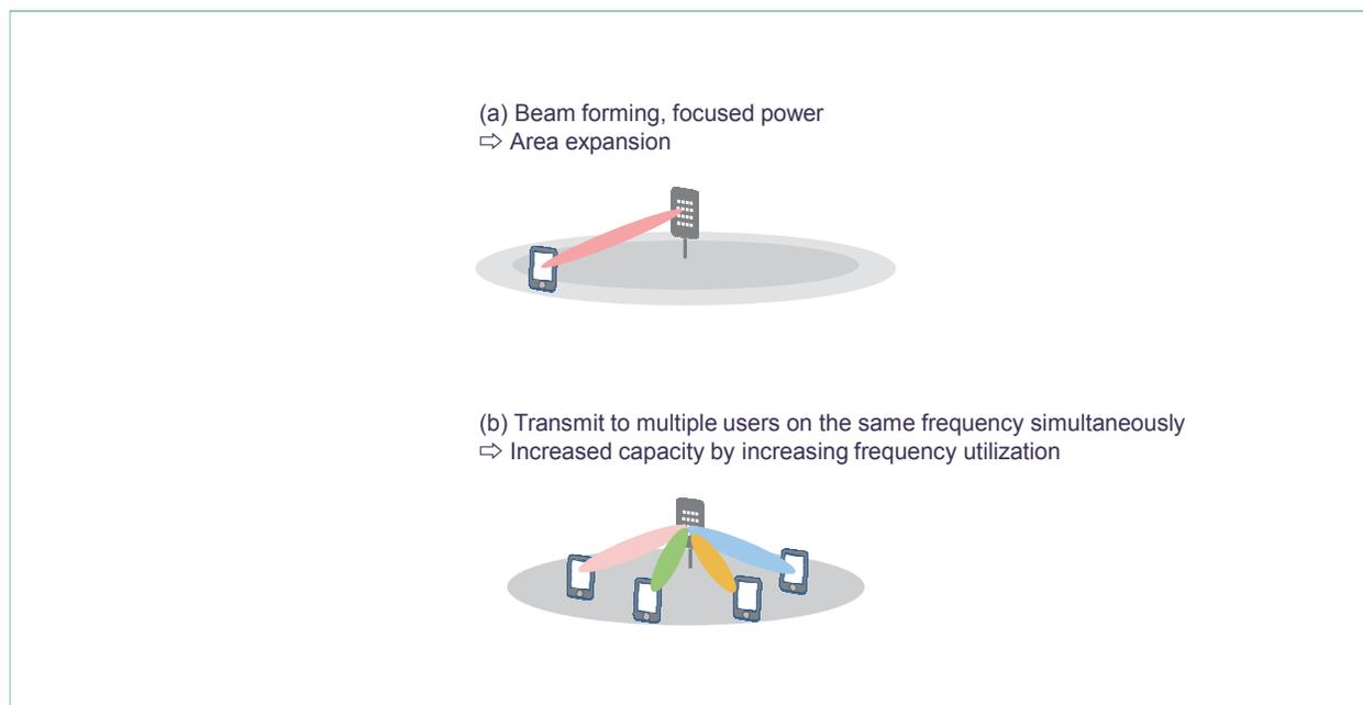
Figure 2 Massive MIMO
