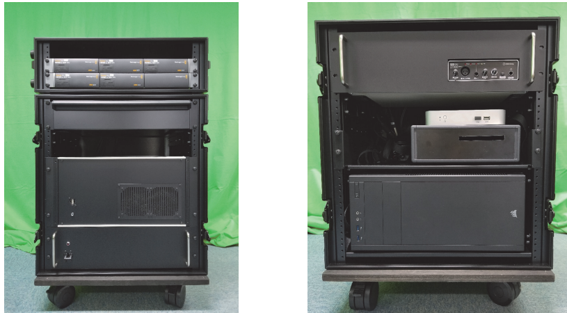
Figure 3 Stitching equipment (left), encoding equipment (right)
