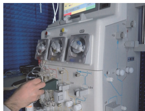
Investigating with a horn antenna
