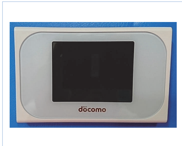
Photo 1 External appearance of router-type mobile terminal supporting 4×4 MIMO
