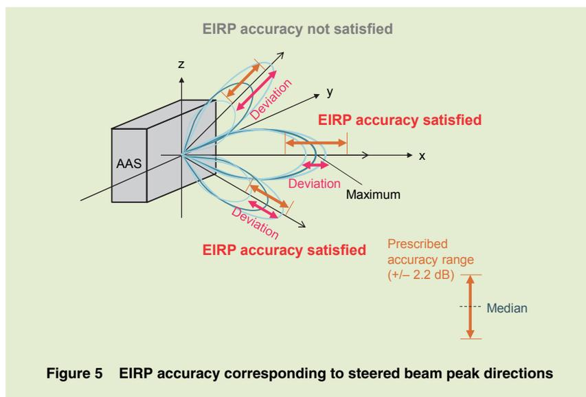
Figure 5 EIRP accuracy corresponding to steered beam peak directions
