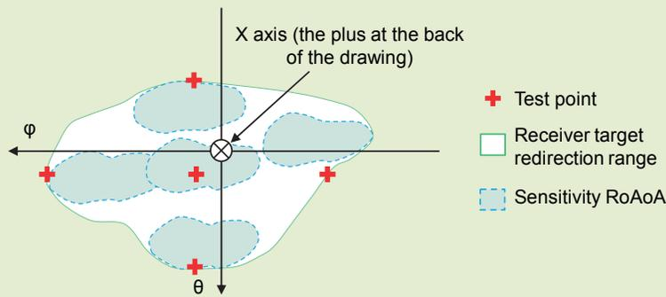
**Figure 7 Range satisfying OTA sensitivity requirements and test points**
