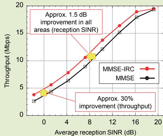
Figure 9 Throughput improvements with the MMSE-IRC receiver
