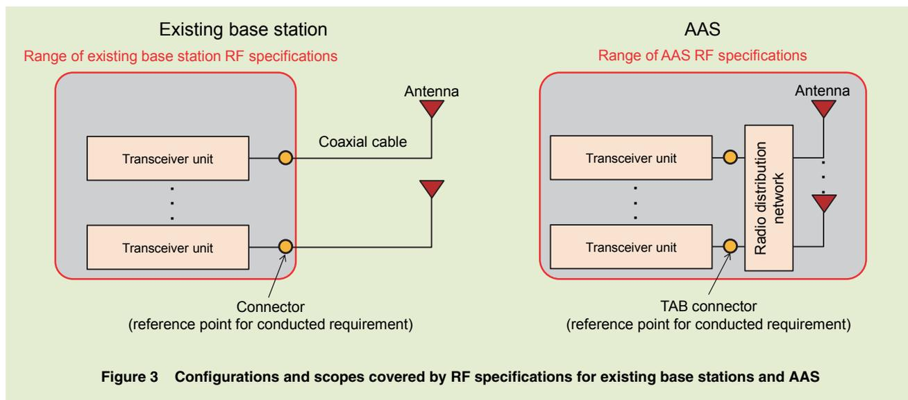
Figure 3 Configurations and scopes covered by RF specifications for existing base stations and AAS
