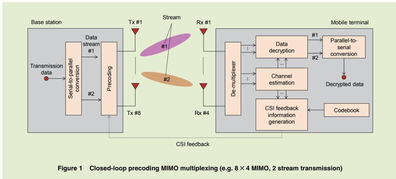
**Figure 1 Closed-loop precoding MIMO multiplexing (e.g. 8 × 4 MIMO, 2 stream transmission)**
