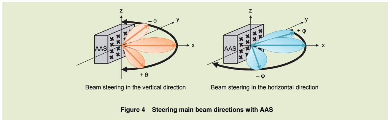
Figure 4 Steering main beam directions with AAS
