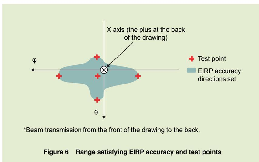
Figure 6 Range satisfying EIRP accuracy and test points
