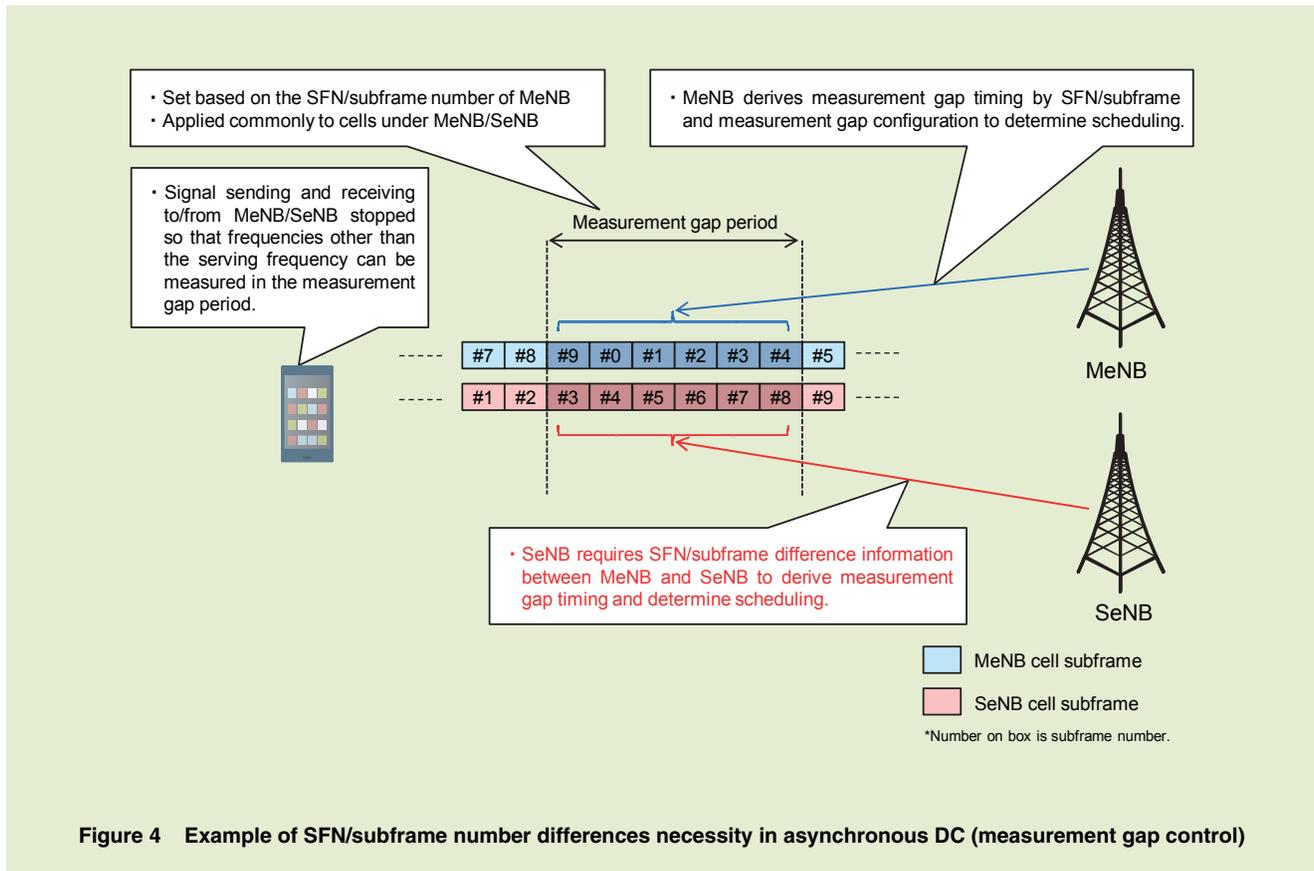
Figure 4 Example of SFN/subframe number differences necessity in asynchronous DC (measurement gap control)
