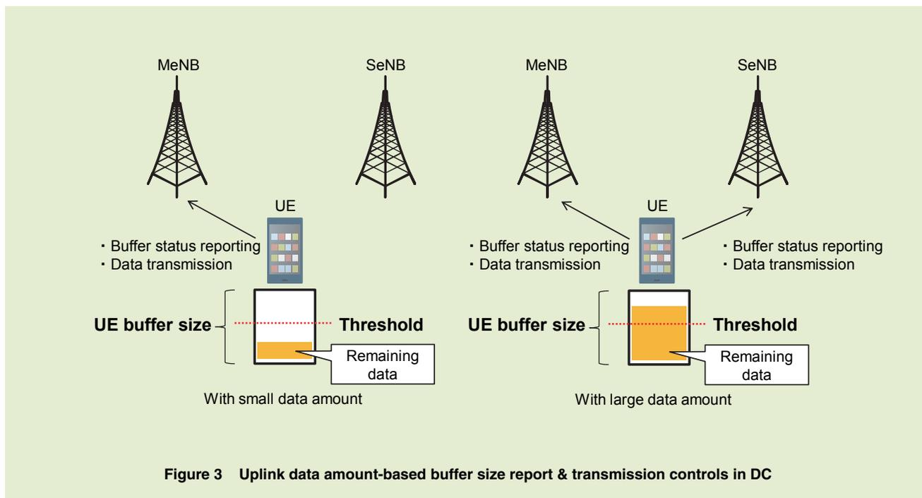
**Figure 3 Uplink data amount-based buffer size report & transmission controls in DC**
