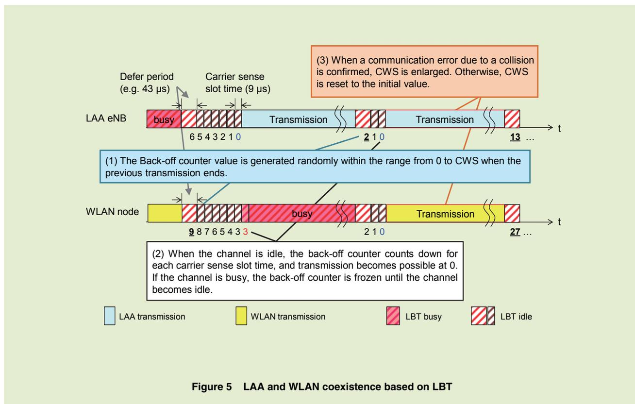
Figure 5 LAA and WLAN coexistence based on LBT
