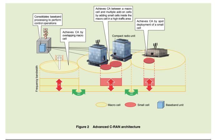
**\*12 HO:** A technology for switching base stations without interrupting communications when a terminal with a call in progress straddles two base stations while moving.
