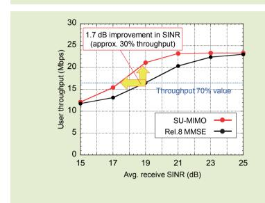
Figure 7 Throughput improvement using a SU-MIMO receiver
