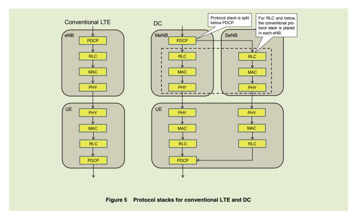
RLC layer down. The UE side has the corresponding protocol layers.
