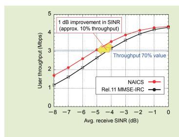
Figure 6 Throughput improvement using a NAICS receiver
