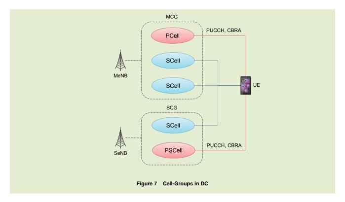
in the PUCCH of the PSCell. In this way, each carrier configured for the UE is associated with a PCell or PSCell, forming a Cell-Group (CG). For this reason, the CG under the MeNB is called a Master Cell-Group (MCG) and a CG under an SeNB is called a Secondary Cell-Group (SCG). MAC layer and physical layer control, such as scheduling, is performed per CG.
