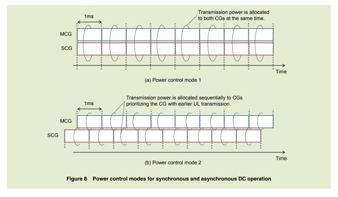
does not assume synchronization between CCs, has been specified. Thus, UE supporting DC is implemented assuming these two types of operations.
