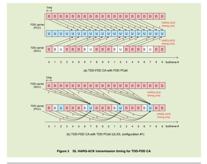
signals for FDD SCells is determined based on the UL/DL configuration of the TDD PCell. Thus, with a TDD PCell, HARQ transmission control for the TDD carrier can be applied to FDD SCells, as if the SCells were TDD carriers.
