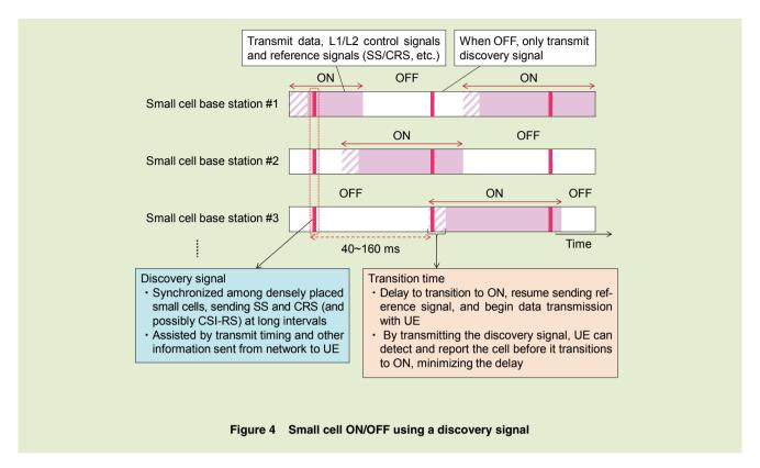
ing the report, the cell can transit to the ON state at an appropriate time, to minimize the transition time before starting communication with the UE. Compared to small cells without ON/OFF switching and discovery signals (i.e., using legacy CRS in every subframe), cells sending discovery signals at long intervals in the OFF state cause much less interference to neighboring cells.
