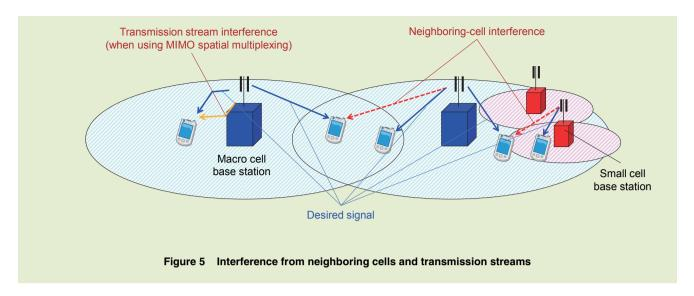
2.1, interference between macro cells and small cells is also expected to become more serious. Although interference from neighboring cells is smaller for UEs near the connected base station, as also shown in Fig. 5, interference between transmission streams will still be an issue, assuming MIMO spatial multiplexing is applied to improve throughput.
