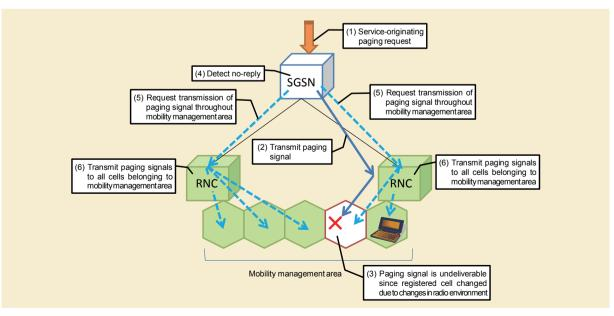
Technology Reports Network Functions Geared to Operating Characteristics of M2M Devices (P.11) Area-limited paging signaling (registered cell changed)
