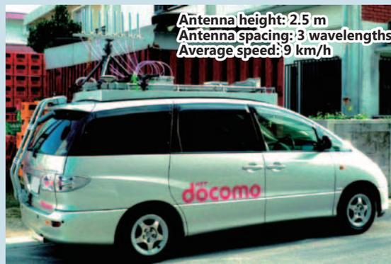
Photo 3 MS with 8-element omnidirectional antenna
