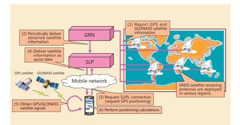
Figure 2 Overview of A-GNSS positioning and network configuration
