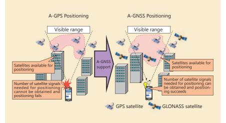
Figure 1 Limits of A-GPS positioning and improvement by A-GNSS positioning
