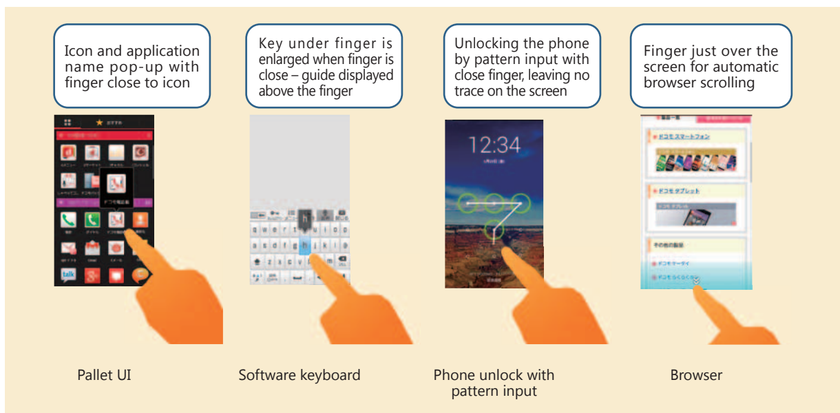
Technology Reports User Operations Assistance Functions Using Finger Proximity Position Information (P.25) Assistance functions using finger proximity position information
