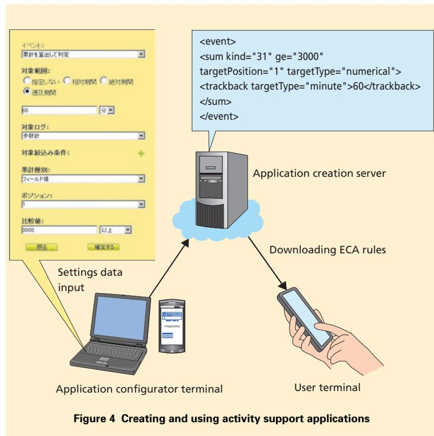
**Figure 4** Creating and using activity support applications
