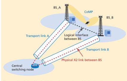
Figure 5 Physical and logical X2 interfaces on the mobile backhaul access network
