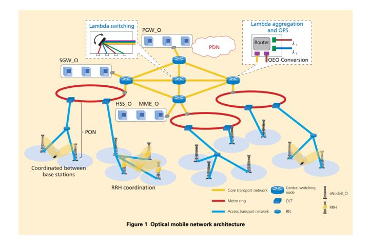
many OEO conversions and electricaldomain processing required for tunnel management and data transport consume energy and introduce delay. As mentioned earlier, reducing the number of OEO conversions and electronic processing in the OMN is an important research topic for DOCOMO Euro-Labs.
