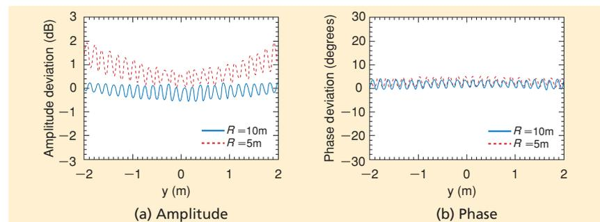
**Figure 4 Electric field distribution around the AUT (applying the proposed method)**
