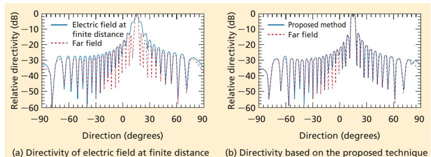
**Figure 2 Results of radiation pattern verification by simulation**
