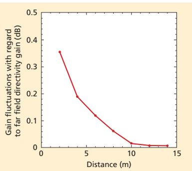
**Figure 6** Variation of gain with measurement distance
