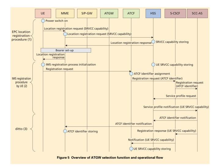
location in the EPC after power activation or any other trigger, it transmits to the MME a location registration request and notifies its SRVCC capability. The MME will store the SRVCC capability information and if there is any change in the capability it will notify the HSS. The HSS will store the SRVCC capability information of the UE and executes tasks such as the eSRVCC application judgment and the notification of the SRVCC capability to the SCC-AS.
