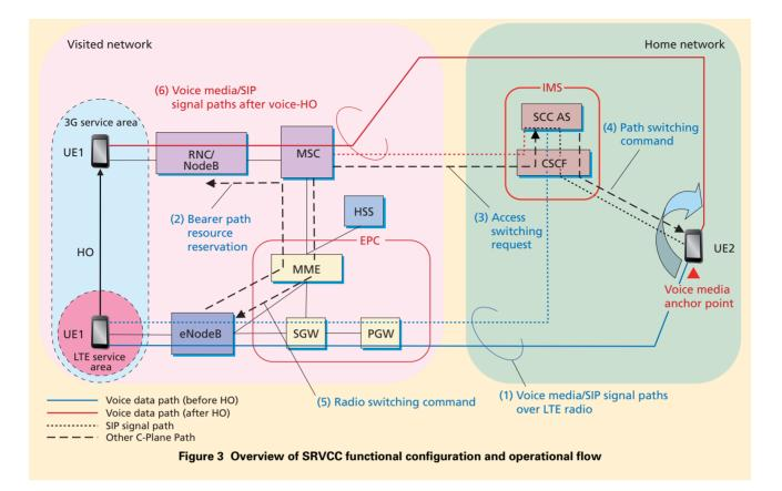
UE2 by means of the IMS. As a result of the call processing, a voice media bearer path is set up in the section links UE1–PGW–UE2 and the sending/receiving of voice data is started between UE1 and UE2 using this path (fig. 3(1)).
