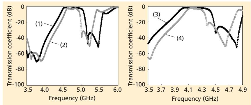
**Figure 4 Tunable BPF frequency characteristics**
