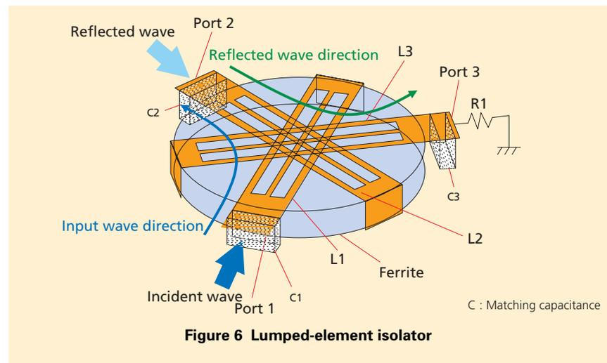
Figure 6 Lumped-element isolator
