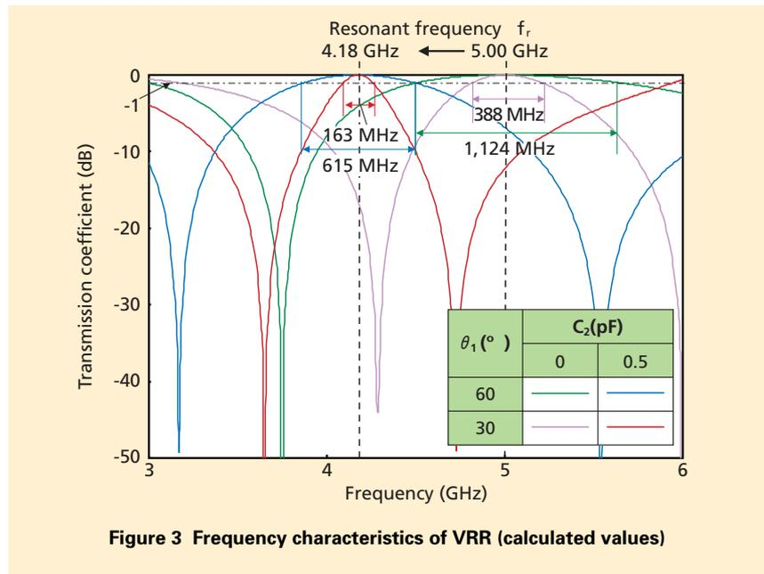
Figure 3 Frequency characteristics of VRR (calculated values)
