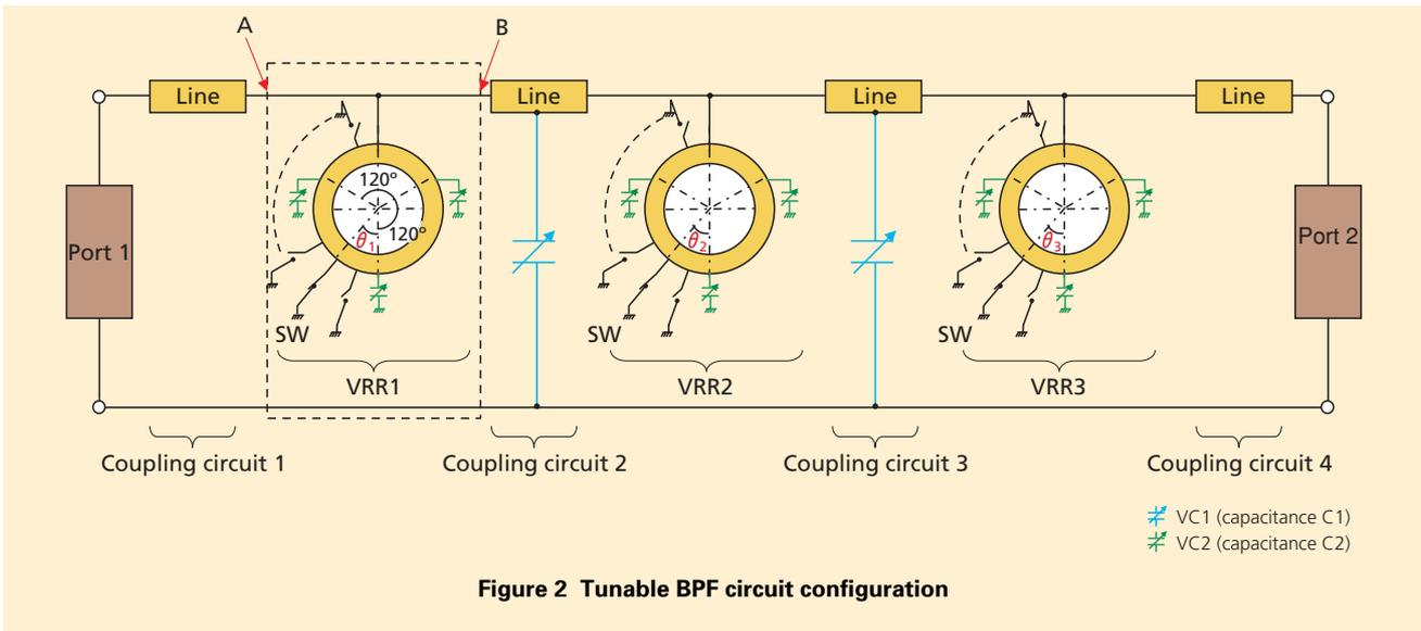
Figure 2 Tunable BPF circuit configuration
