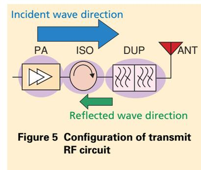
Figure 5 Configuration of transmit RF circuit
