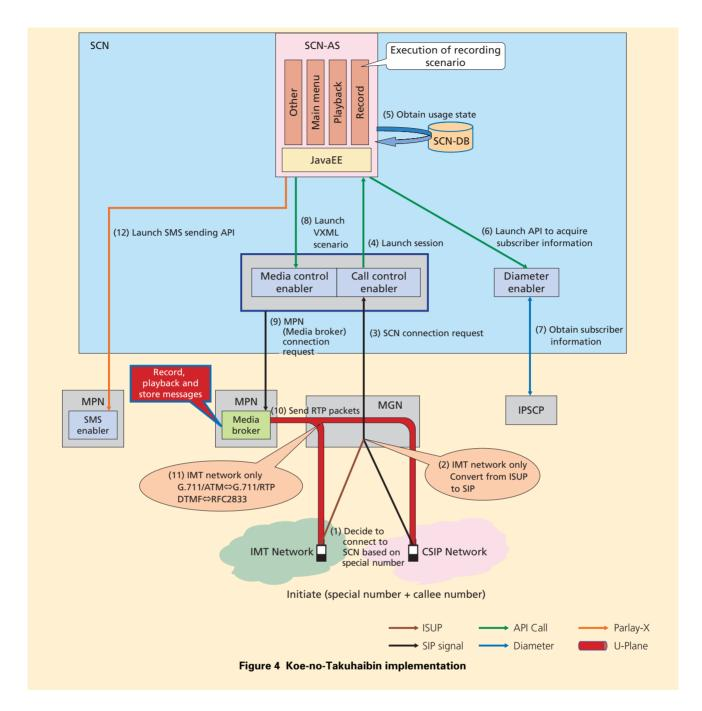
charges from the contract information, and then launches a VXML <sup>\*38</sup> scenario with the call control enabler and media control enabler (Fig. 4 (8)). The mashup API for call control and media control is launched, a connection to the media broker<sup>\*39</sup> (MPN) is requested in order to connect in the U-plane and send guidance for recording (Fig. 4 (9)), and sessions are established between
