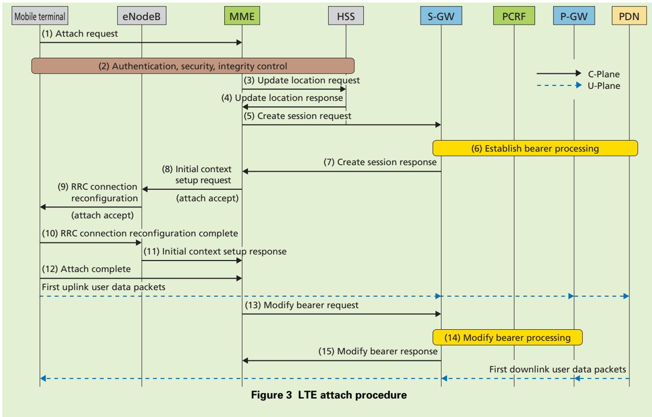
Figure 3 LTE attach procedure
