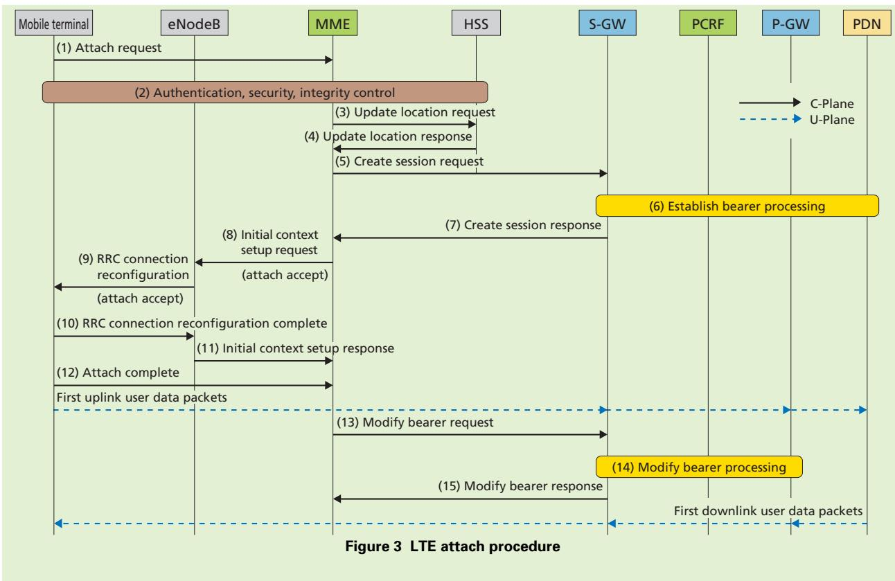
**Figure 3 LTE attach procedure**
