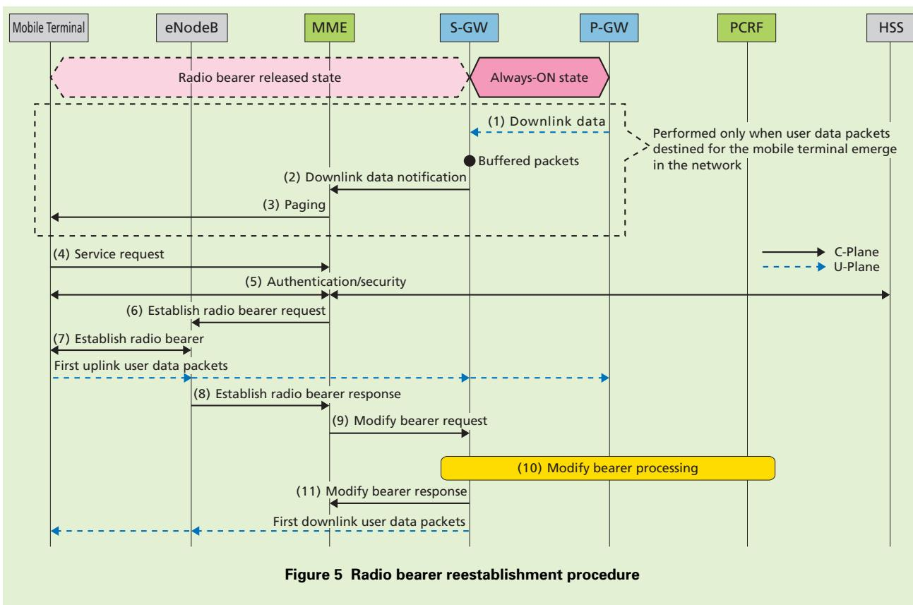
Figure 5 Radio bearer reestablishment procedure
