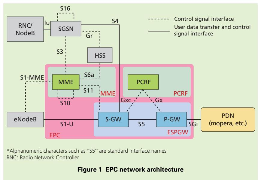
\*5 **SGSN:** A logical node having packet communication functions specified by 3GPP standards.
