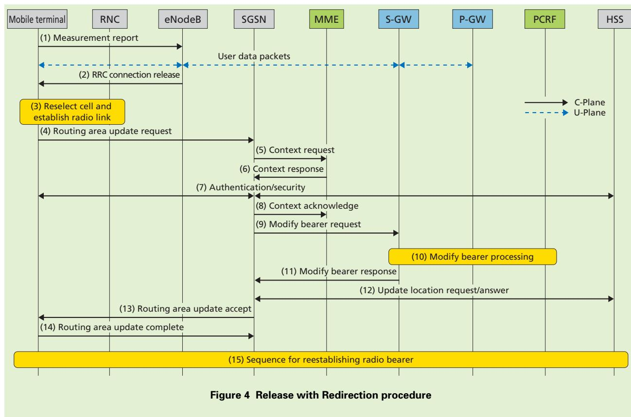
**Figure 4 Release with Redirection procedure**
