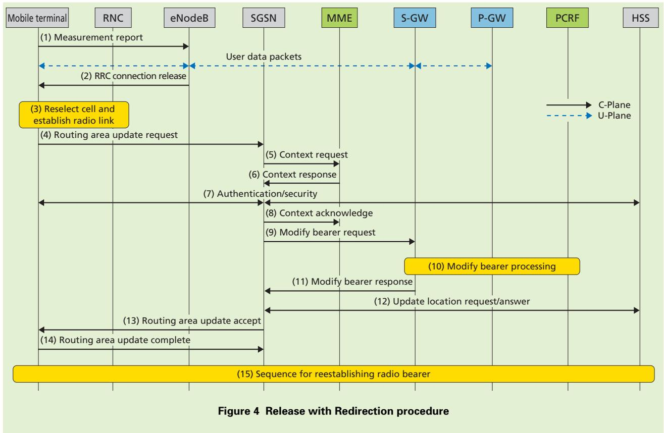
Figure 4 Release with Redirection procedure
