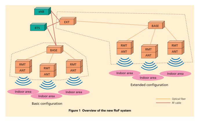
\*1 Transmit diversity: Technology which utilizes the differences in channel fluctuation between transmission antenna channels to obtain diversity gain. fiber. Up to 256 remote units can be connected to a single BASE unit. Also able to supply power to each of the remote units.
