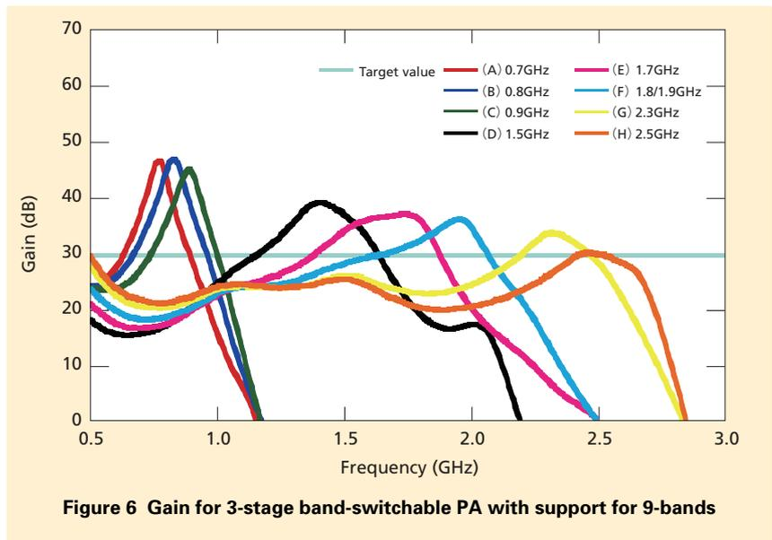
**Figure 6 Gain for 3-stage band-switchable PA with support for 9-bands**
