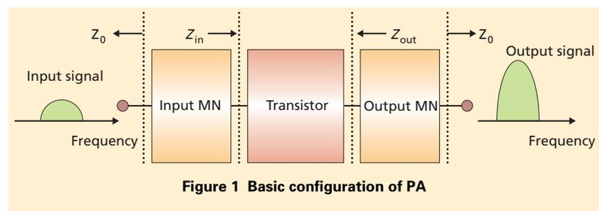
Figure 1 Basic configuration of PA
