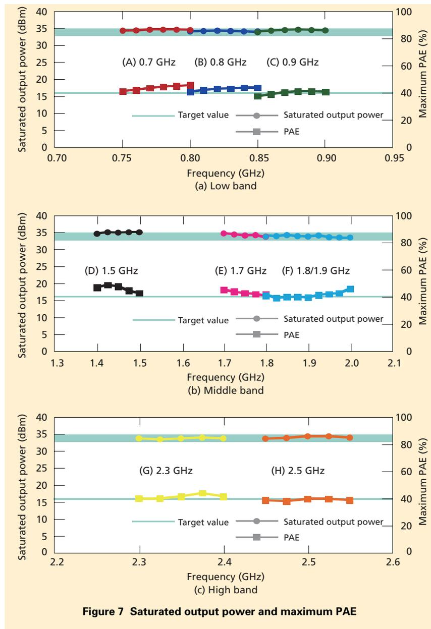
Figure 7 Saturated output power and maximum PAE
