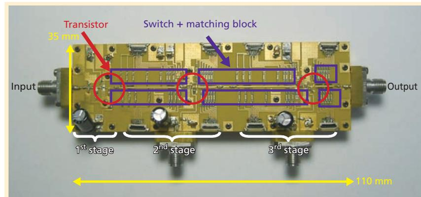
**Photo 1 3-stage band-switchable PA with support for 9-bands**
