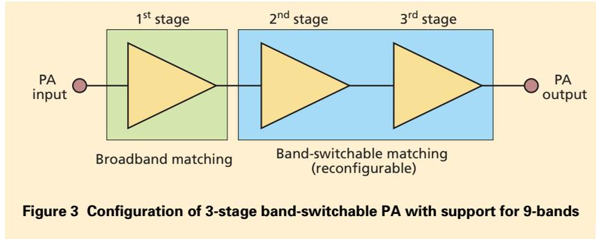
**Figure 3 Configuration of 3-stage band-switchable PA with support for 9-bands**
