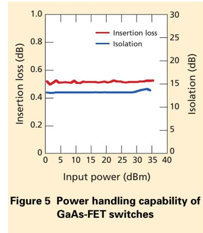
**Figure 5 Power handling capability of GaAs-FET switches**
