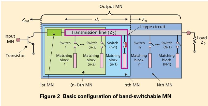
Figure 2 Basic configuration of band-switchable MN
