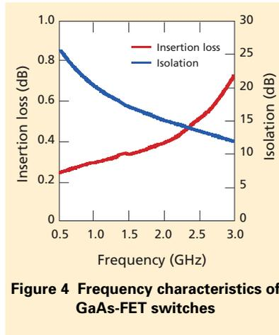
**Figure 4 Frequency characteristics of GaAs-FET switches**
