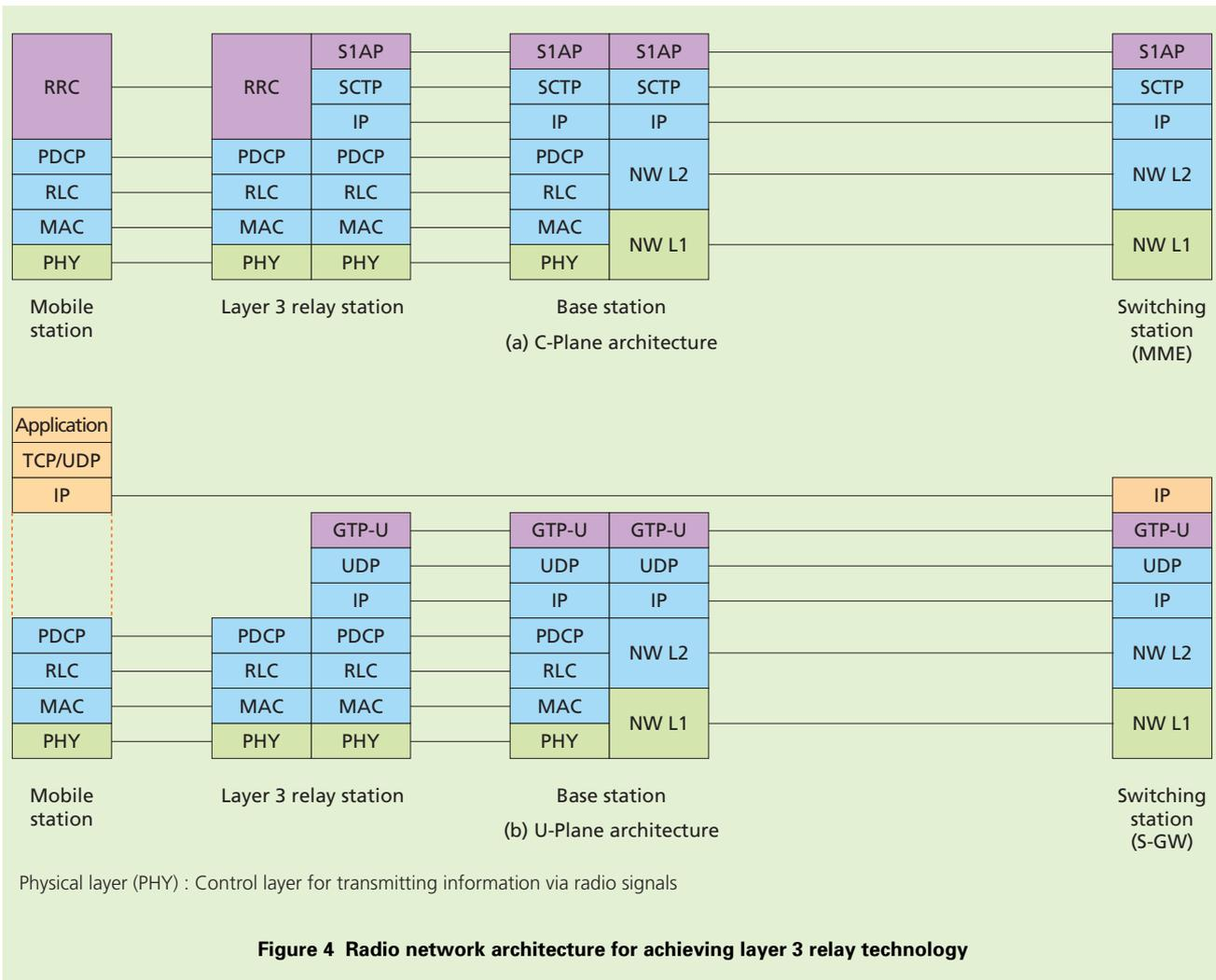
Figure 4 Radio network architecture for achieving layer 3 relay technology
