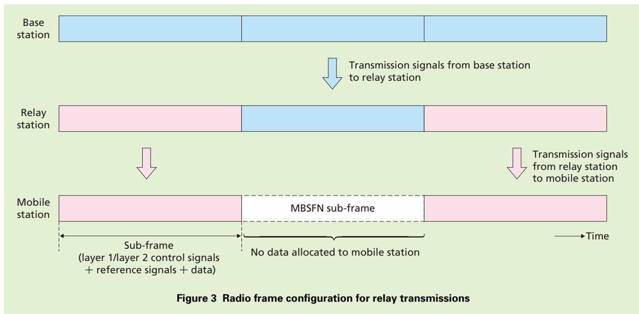
Figure 3 Radio frame configuration for relay transmissions
