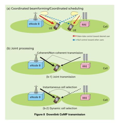
cell selection, in which cells can be selected at any time in consideration of interference, are being studied. For joint transmission, two methods are being studied: non-coherent transmission, which uses soft-combining reception of the OFDM signal; and coherent transmission, which does precoding between cells and uses in-phase combining at the receiver.
