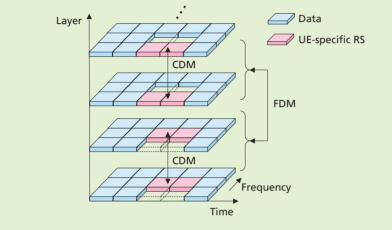
Figure 4 UE-specific RS multiplexing
