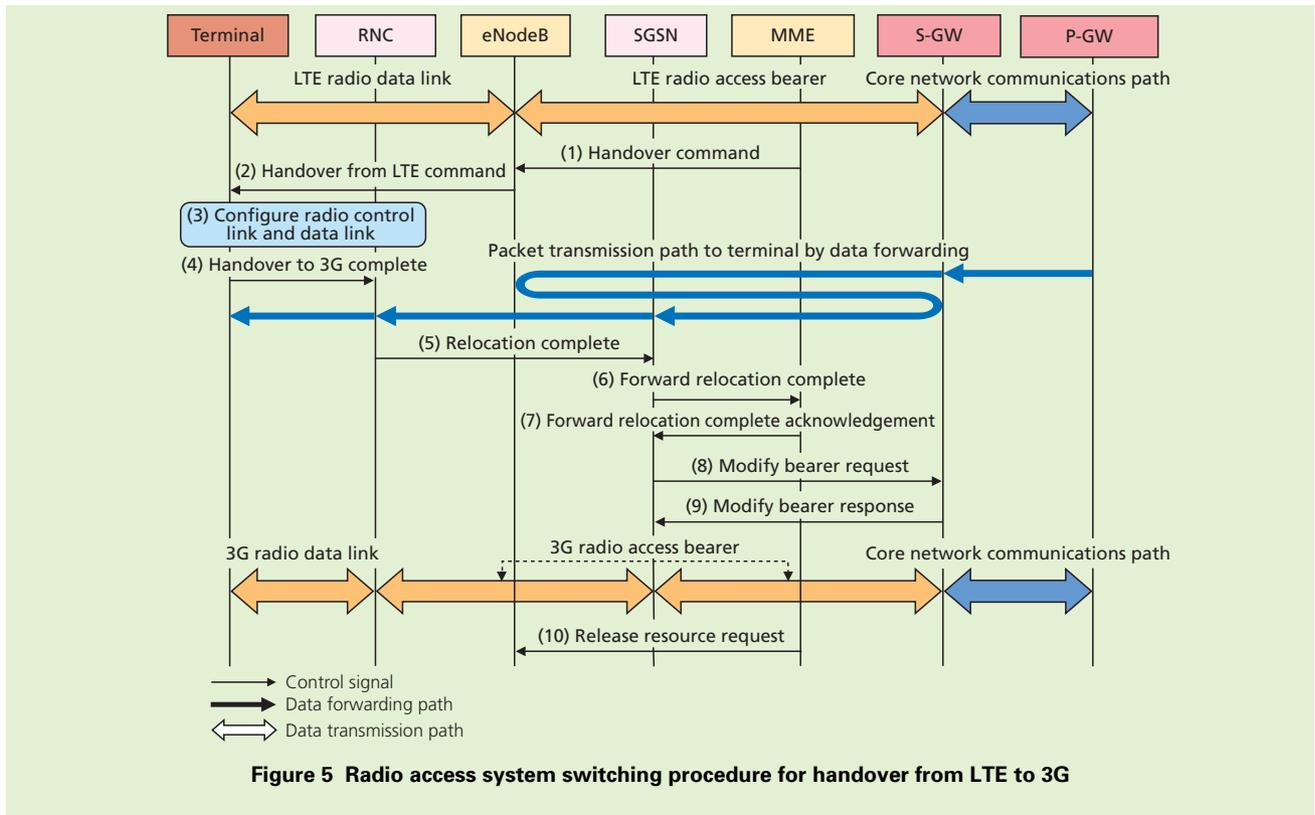
Figure 5 Radio access system switching procedure for handover from LTE to 3G
