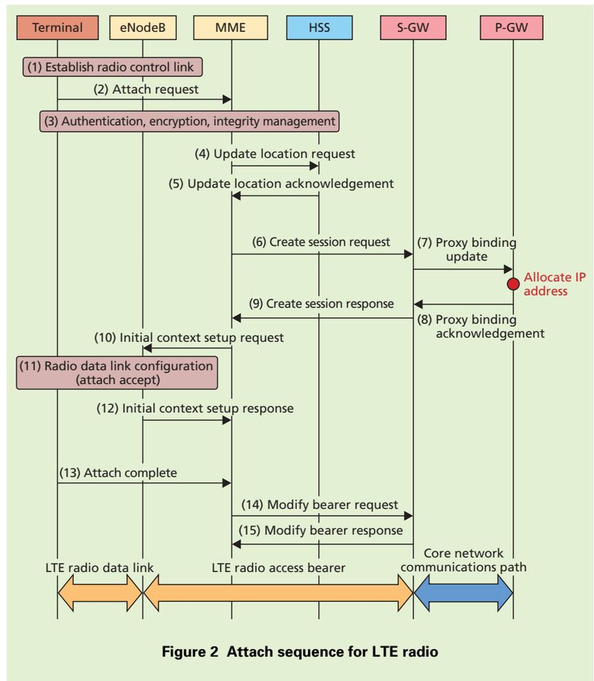
Figure 2 Attach sequence for LTE radio
