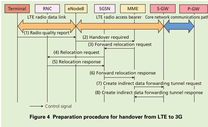
other information it received from the eNodeB to the SGSN in a forward relocation<sup>\*12</sup> request signal. The information required to configure the communications path between the S-GW and SGSN, which is used for data transmission after the MME has completed the handover, is sent at the same time.
