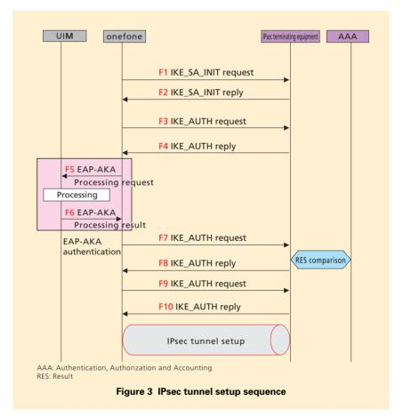
ing IKE\_AUTH message exchange the information for establishing the IPsec tunnel.
