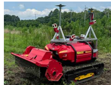
Autonomous undergrowth-clearing machine equipped with a high-precision positioning satellite system
