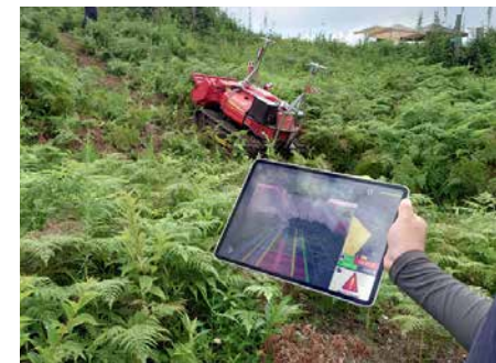
Capable of climbing slopes of approximately 25 degrees and of driving and mowing on slopes of up to 45 degrees
