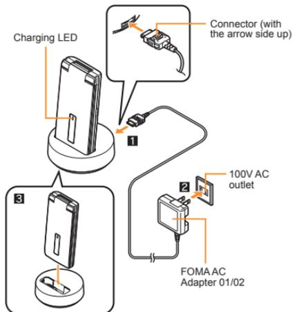
**4 When charging is complete, the charge alert is heard and the charging LED turns off**
